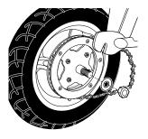
**5** Pull the wheel out. Note the arrangement of the hardware sequence.
